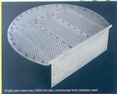
Single pass sieve tray (1600 mm dia.) constructed from stainless steel
